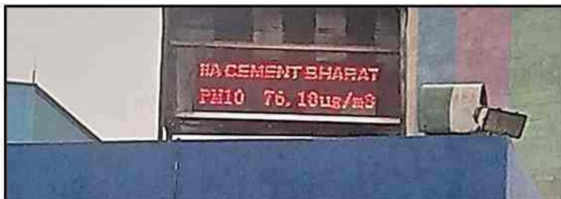
Display board of real time ambient air quality installed at factory main gate
